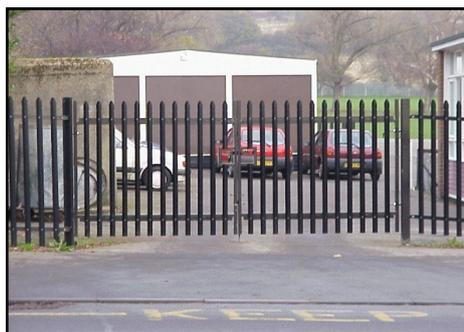
**Posts** - 100mm x 55mm RSJ or 102mm x 44mm RSJ or 127mm x 76mm RSJ depending on height of the fence. Posts installed at 2.75m centres.
